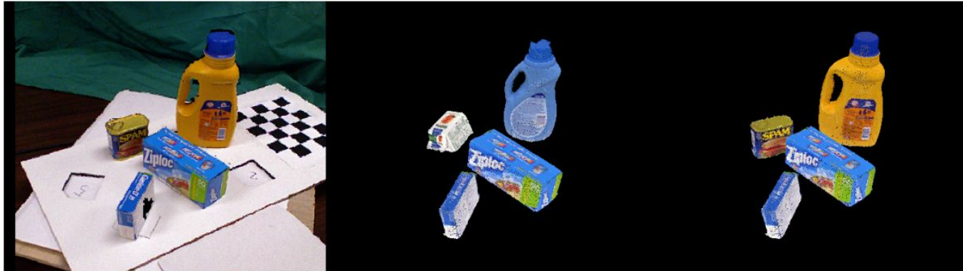
Fig. 7. Object recognition and pose estimation example: input scene (left), results obtained using ESF (center) and GASD-SI (right).
